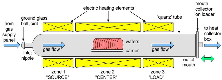
3-zone tube furnaces are most common, but 5-zone tube furnaces also exist.
