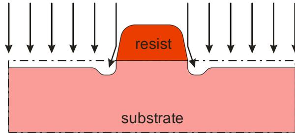
Trenching of substrate occurs adjacent to resist edges.
